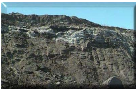
Overburden Waste Pile Sits Atop An Oil Sands Open Pit Surface Mine
